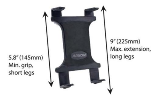
Slim Grip Universal Tablet Holder allows a maximum extension up to 9'' (225mm), and a minimum grip of 5.8'' (145mm).
